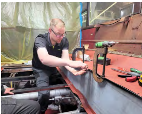
Connor Drage busy at work on the long bench seat support panels above Newcastle 628's rear wheel arch. [Connor Drage]
