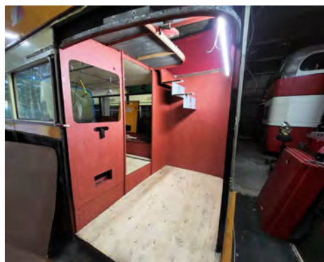
628's rebuilt rear platform and entrance to the lower saloon. [Connor Drage]
