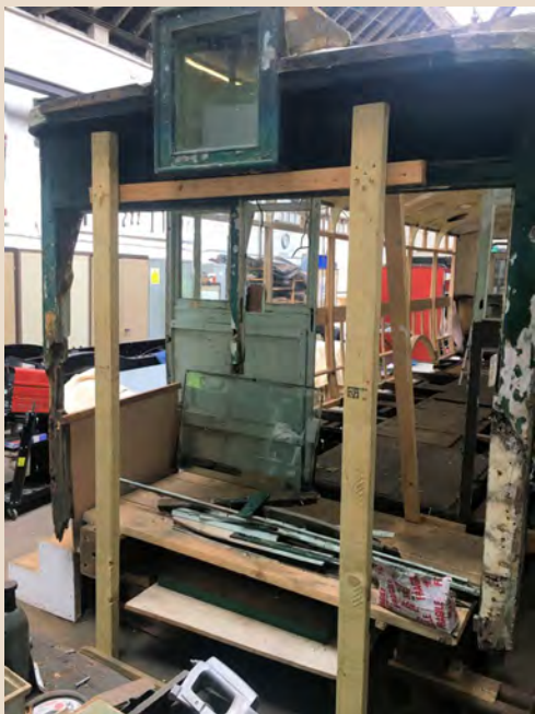
Lower right: Rebuilding the front end.
