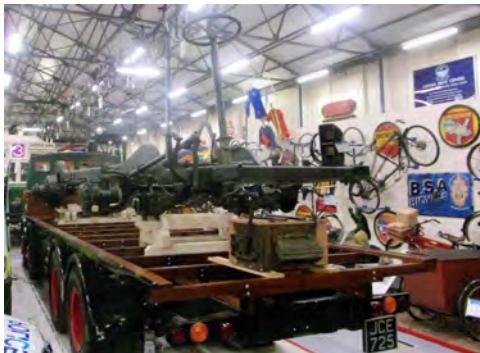
The chassis of Ipswich 16, built locally by Ransomes, Sims and Jefferies in 1926, which originally carried a R, S&J body, is displayed on the back of a lorry. [Simon Guppy]
